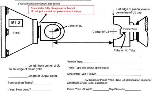
Note: OE Ford 8" and 9" Pinion yokes can use either a 1 1/16 or 1 1/8 cap diameter. This is only 1/16 different but is critical that this is checked carefully. Call if if you have any question on this.
