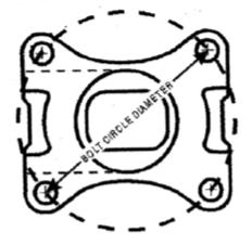
We may need bolt circle diameter. We may need a length from top to bottom of holes and left to right to determine bolt pattern.
